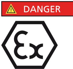
The temperature class specifies the maximum permissible temperature at the surface of the pump set during operation. For the permissible operating temperature of the pump in question refer to the data sheet.
