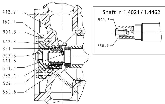
**Fig. 25:** Dismantling the plain bearing - radial suction nozzle
