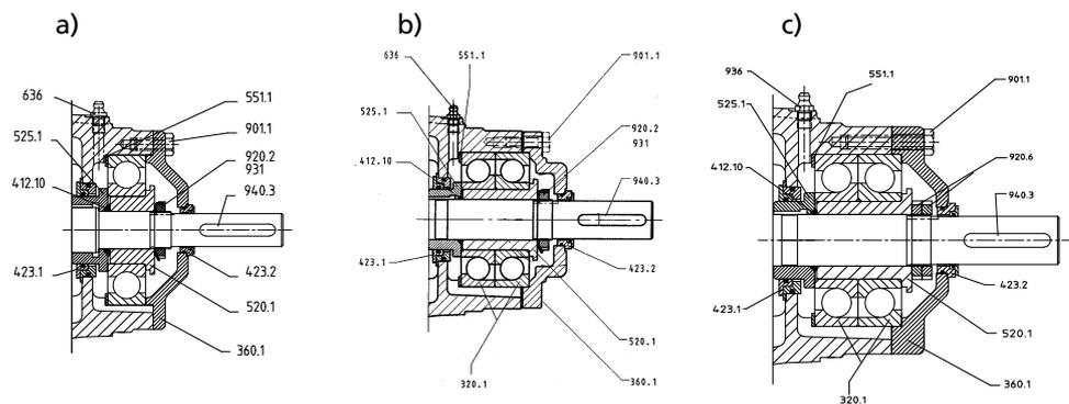
**Fig. 32:** Grease lubrication with labyrinth seal: a) size 32 and b) sizes 50-65 and c) size 100-200
