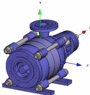
Fig. 9: Forces and moments at the pump nozzles
