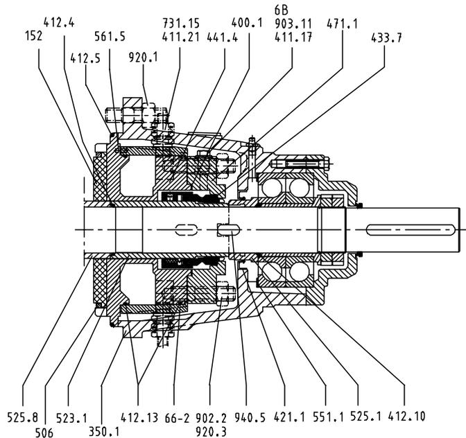
**Fig. 38:** Removing a water-cooled mechanical seal
