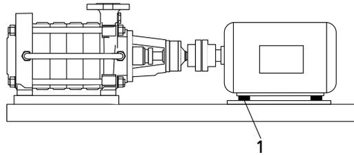
**Fig. 16:** Pump set with shims
