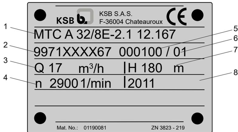
Fig. 5: Name plate (example) of Multitec
