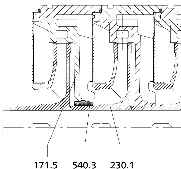
**Fig. 43: Bush (intermediate bearing)**
