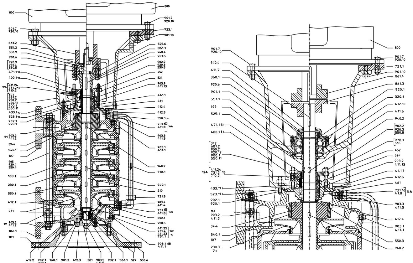
Fig. 62: Installation type V – a) size 32-65 – b) size 100-200
