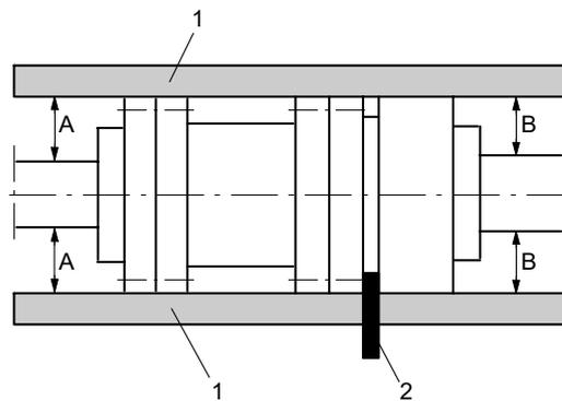
**Fig. 13:** Spacer-type coupling, checking the coupling alignment
