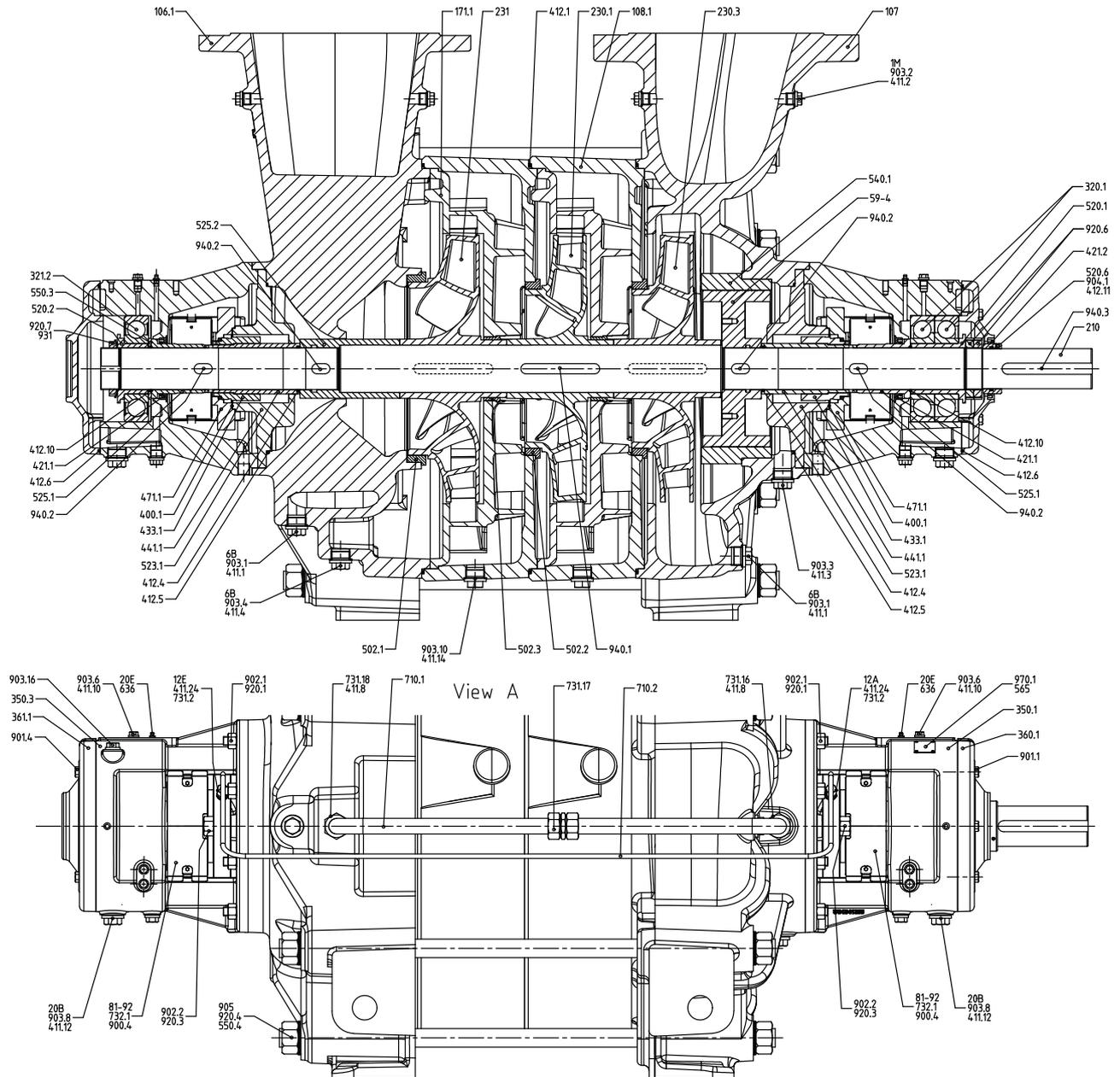
Fig. 60: Installation type C – Multitec 250
