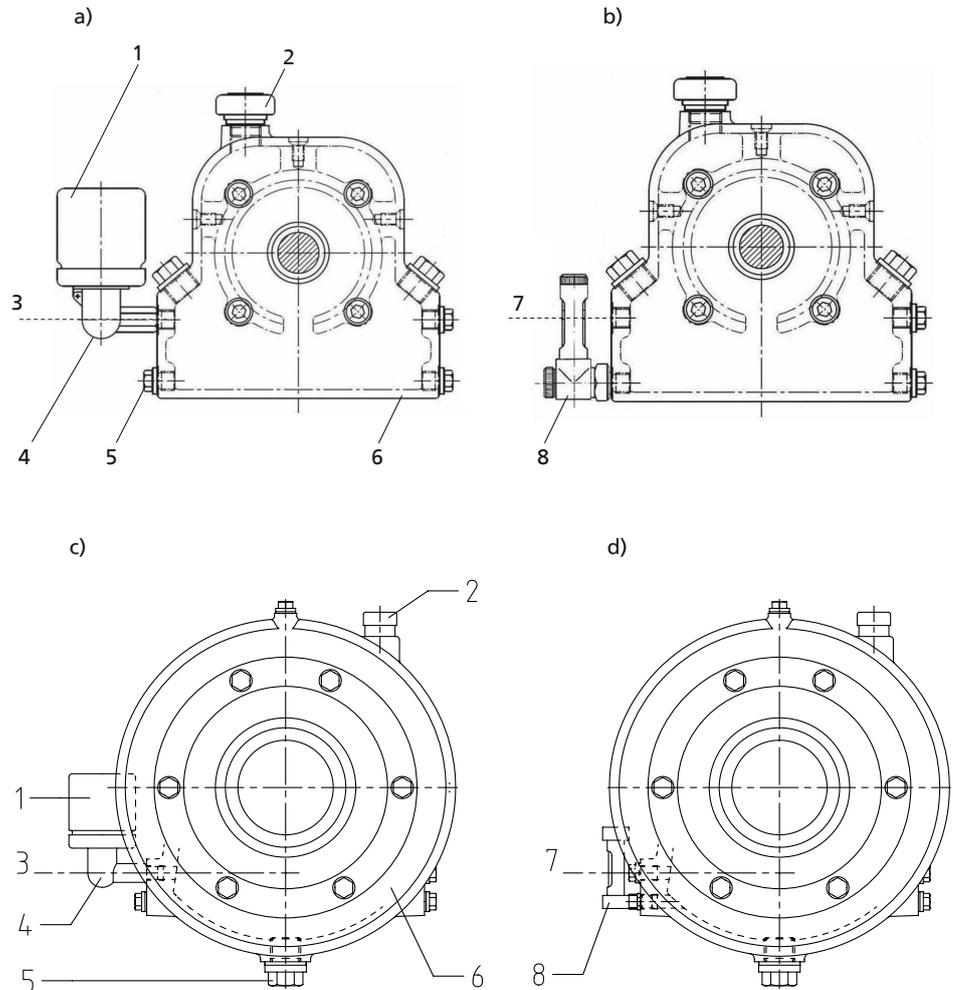
**Fig. 22:** a) Bearing bracket with constant level oiler – b) Bearing bracket with oil level gauge – c) Bearing bracket with constant level oiler (size 250) – d) Bearing bracket with oil level gauge (size 250)
