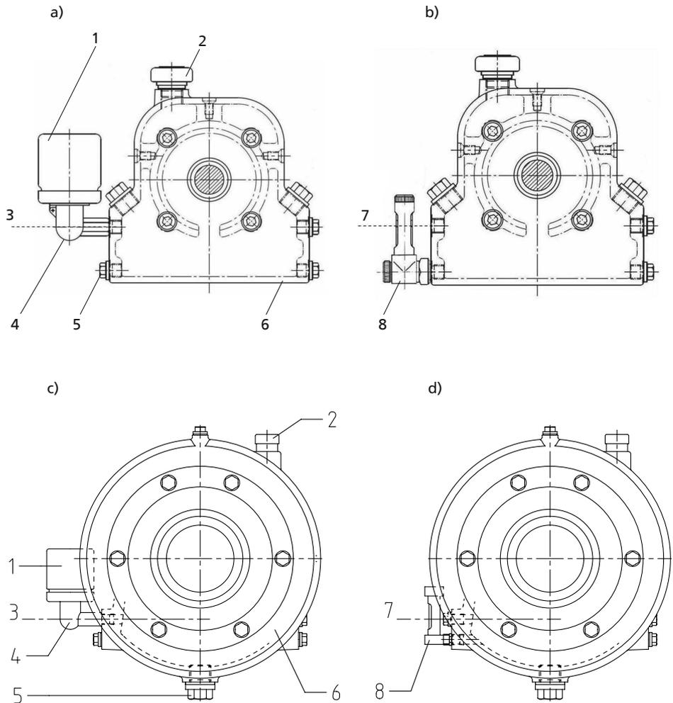
**Fig. 18:** a) Bearing bracket with constant level oiler – b) Bearing bracket with oil level gauge – c) Bearing bracket with constant level oiler (size 250) – d) Bearing bracket with oil level gauge (size 250)
