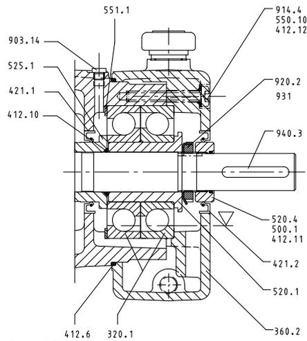
Fig. 50: Oil-lubricated bearings
