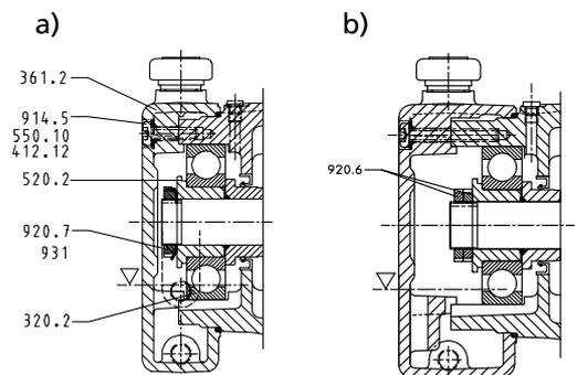
Fig. 29: Oil lubrication with lip seal: a) Multitec 32-125 and b) Multitec 150-200
