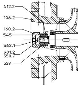
**Fig. 24:** Dismantling the plain bearing - axial suction nozzle
