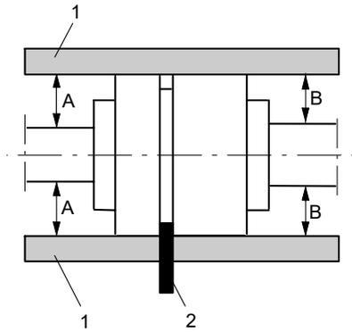
**Fig. 12:** Non-spacer-type coupling, checking the coupling alignment
