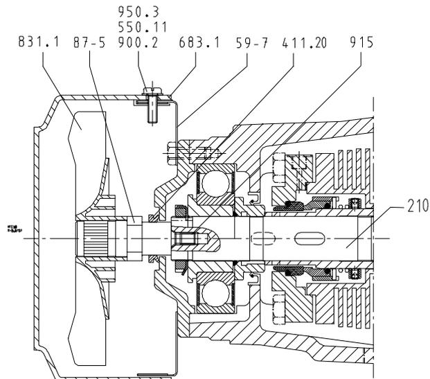
**Fig. 36:** Removing an air-cooled mechanical seal - additional dismantling steps
