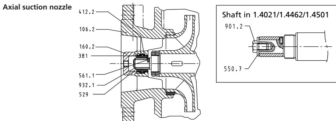
**Fig. 23:** Dismantling the plain bearing - axial suction nozzle
