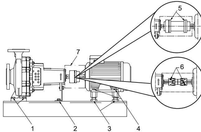
**Fig. 26:** Position of bolts/screws at the pump set
