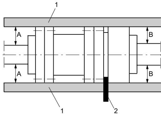
Fig. 14: Spacer-type coupling, checking the coupling alignment
