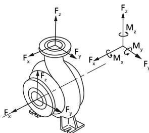
**Fig. 10:** Forces and moments at the pump nozzles
