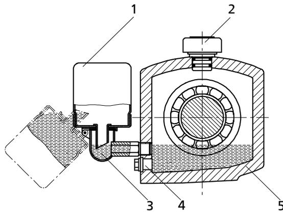
**Fig. 18:** Bearing bracket with constant level oiler
