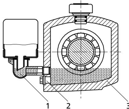
Fig. 19: Bearing bracket with constant level oiler
