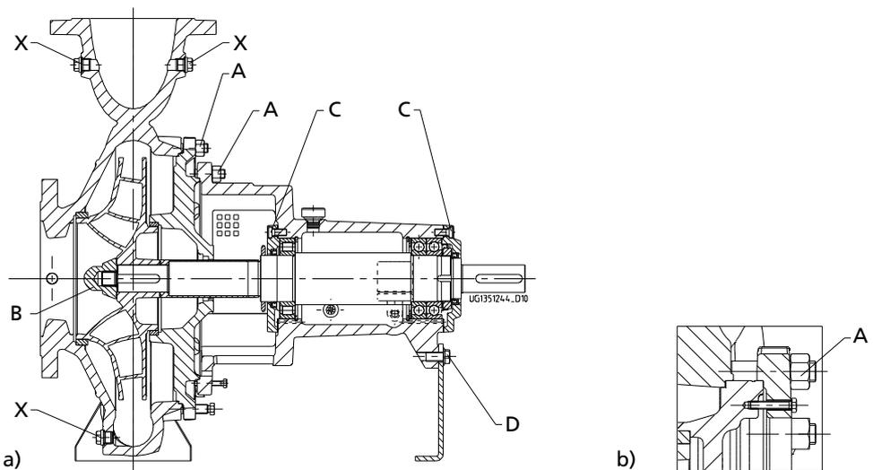
Fig. 23: a) Tightening points at the pump, b) Version with clamped casing cover
