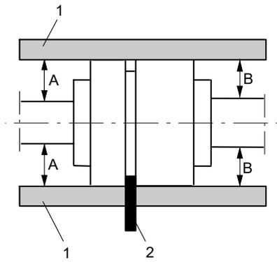
Fig. 13: Non-spacer-type coupling, checking the coupling alignment
