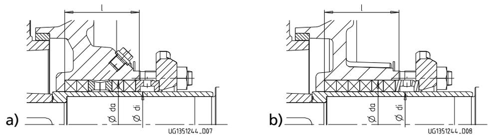
Fig. 22: Gland packing chamber a) with lantern ring and b) without lantern ring
