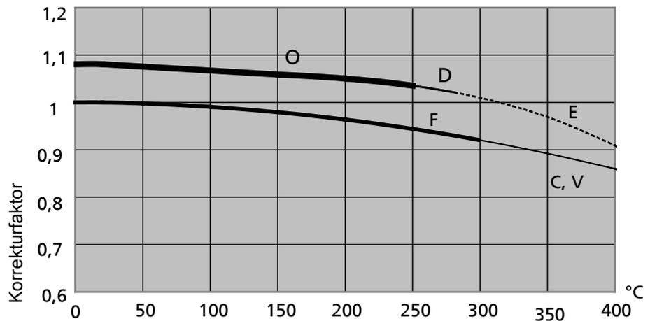
Fig. 11: Temperature correction diagram for "C, D, E, F, V, O variants" (1.4408 / A743 Gr. CF8M)
