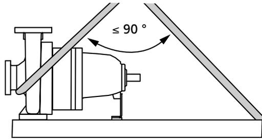
Fig. 4: Transporting the pump on the baseplate
