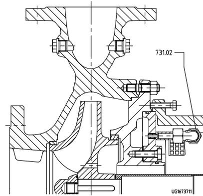
Heatable version, only casing cover cooled/heated
