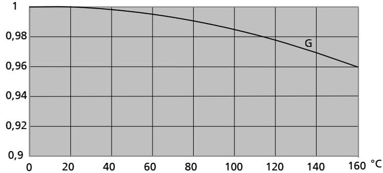
Fig. 12: Temperature correction diagram for material variant G (JL1040/ A48CL35B)
