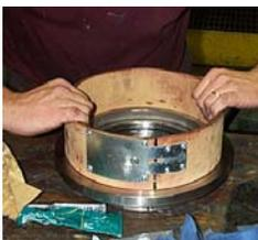
Place the housing end cover and seal holder on a flat, clean surface. Verify that the grooves are clean and free from burrs or sharp edges. Using the correct Seal Installation Tool, locate the machined ridge in the tool over the toric and clamp together. Align the parts squarely with the groove and carefully snap the seal assembly into place using a rapid, even push. Isopropyl alcohol can be used as a lubricant. Allow time for the assembly lube to evaporate.
