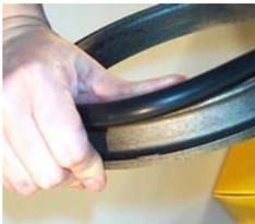
Gently stretch the toric over the metal seal rings until it seats in the radius. Verify that the toric is not twisted by inspecting the mold flash line on the outside diameter. Eliminate any irregularity by gently pulling a section of the toric radially off the ring and letting it snap back. Twisted torics will cause nonuniform face load, resulting in leakage and bearing contamination.
