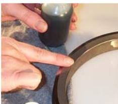
Apply a very thin film of pure Molybdenum Disulfide lubricant or light oil to the seal faces just prior to final assembly. This will lubricate the seals during initial start up. Do not get any lube on the rubber toric rings. Be sure there is no debris on either of the seal faces, since even a small piece of lint can hold the seal faces apart and cause leakage or damage to the sealing surfaces.
