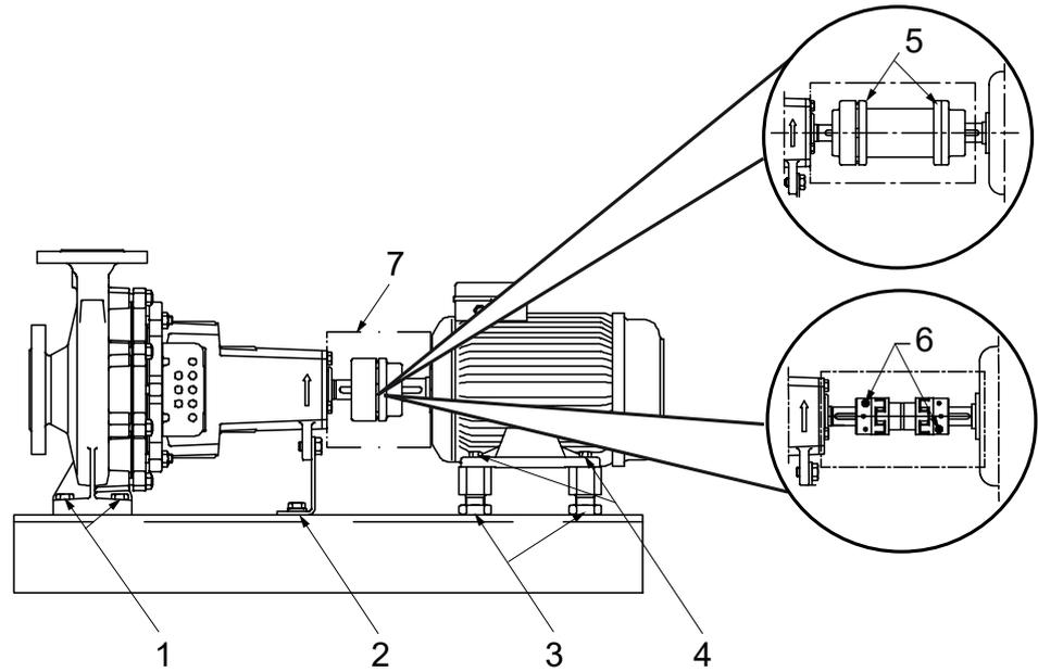
Fig. 19: Tightening points at the pump set
