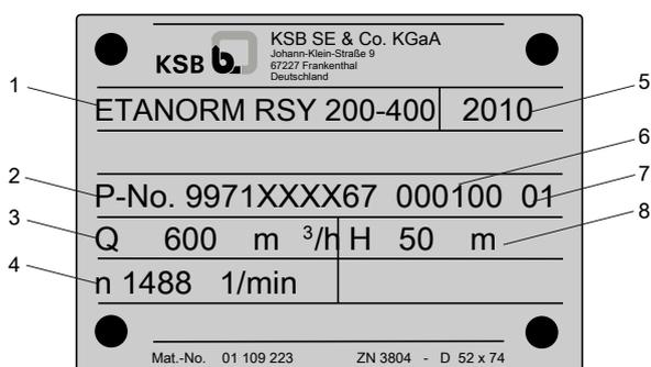
Fig. 5: Name plate (example) Etanorm-RSY
