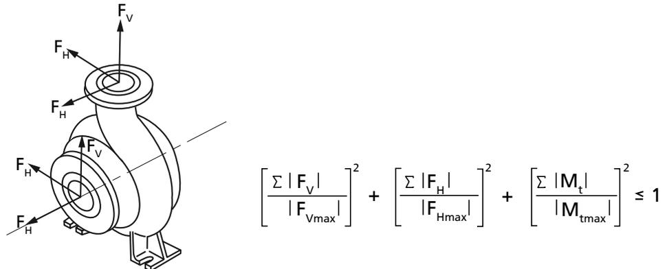
**Fig. 10:** Forces and moments at the pump nozzles
