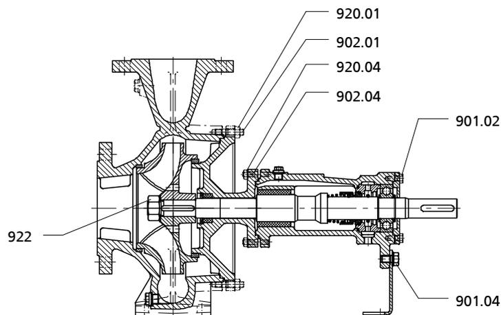
Fig. 18: Tightening points at the pump
