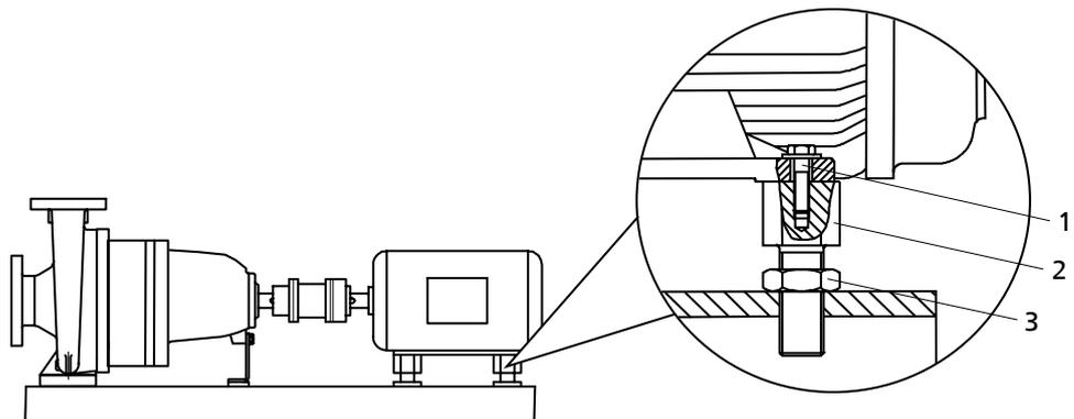
**Fig. 15:** Motor with adjusting screw
