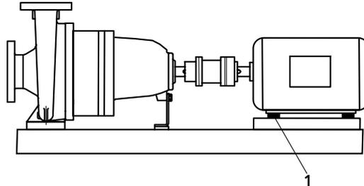
Fig. 16: Pump set with shim
