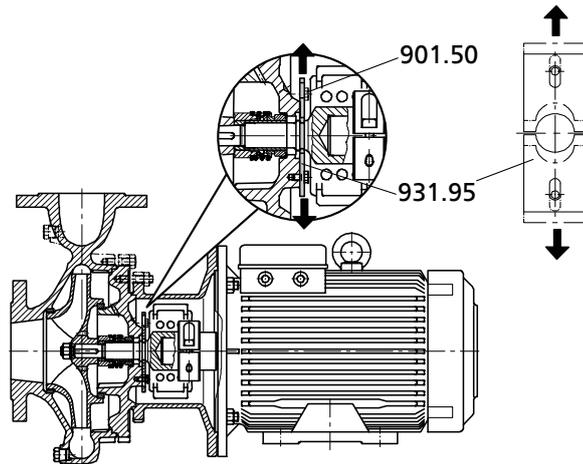
**Fig. 12:** Removing the lock washers
