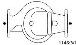
**Fig. 17:** Horizontal installation (for example under the ceiling)
