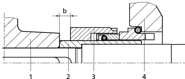
**Fig. 10:** Installation dimension  $b$  of mechanical seal
