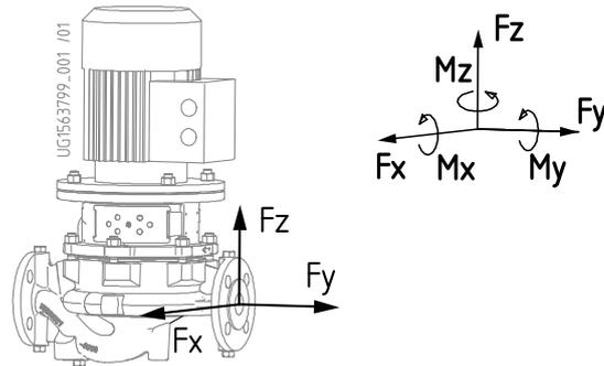
Fig. 8: Forces and moments at the pump nozzles
