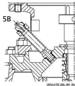
**Fig. 23:** Vent, mechanical seal chamber
