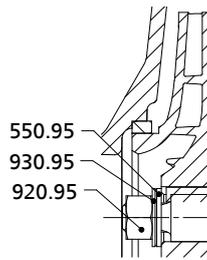
Fig. 30: Fastening elements for the impeller, WS 25
