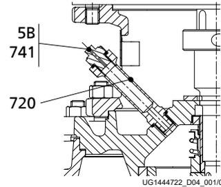
Fig. 31: Vent valve 5B for vertical installation
