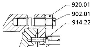
Fig. 32: Fastening elements for the clamped casing cover
