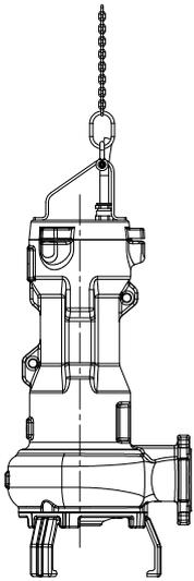
Fig. 16: Attaching the lifting chain / lifting rope
