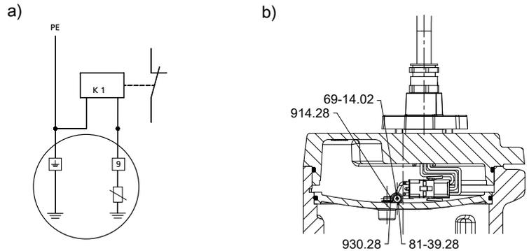
**Fig. 18:** Wiring of the electrode relay: a) Connection diagram, b) Position of the electrode in the motor housing
