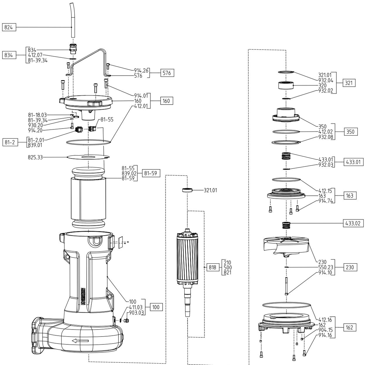
Fig. 32: Exploded view of Amarex D-max, version US
