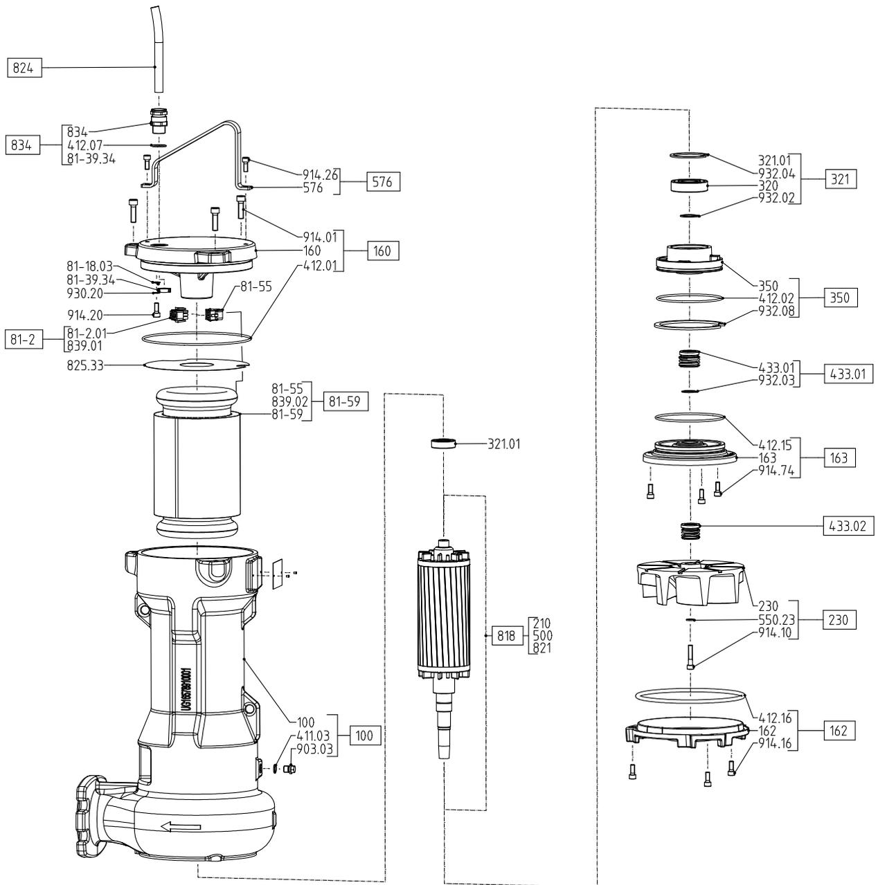
Fig. 31: Exploded view of Amarex F-max, version US
