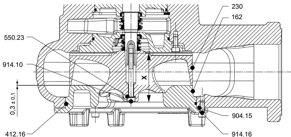
Fig. 25: Fitting the impeller, example impeller type D-max
