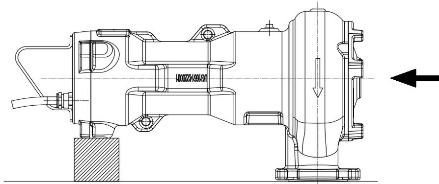
**Fig. 3:** Checking the direction of rotation
