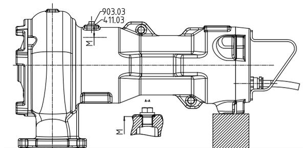
**Fig. 22: Lubricant level**
