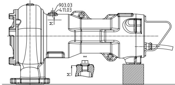
Fig. 2: Lubricant level
