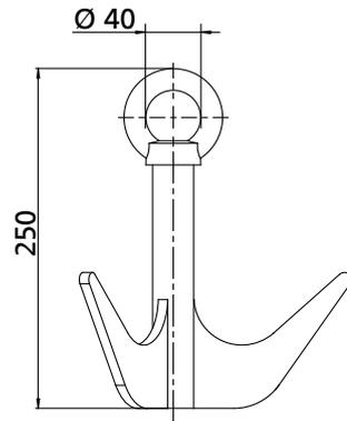
**Fig. 1:** Lifting hook
