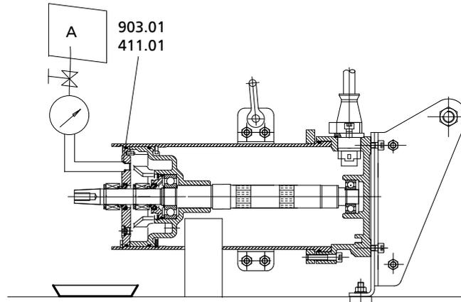
**Fig. 15: Pressure connection**
