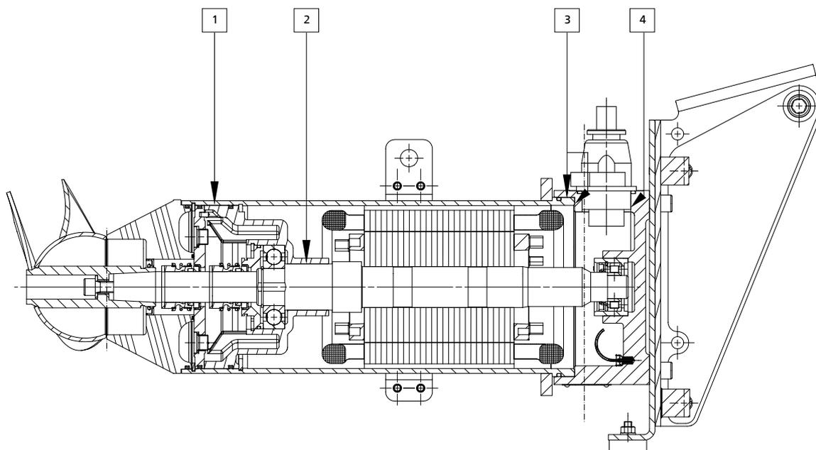
Fig. 21: Flamepaths on explosion-proof motors - Variant C
