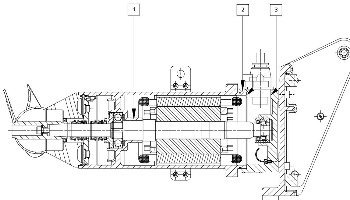
Fig. 22: Flamepaths on explosion-proof motors - Variant G
