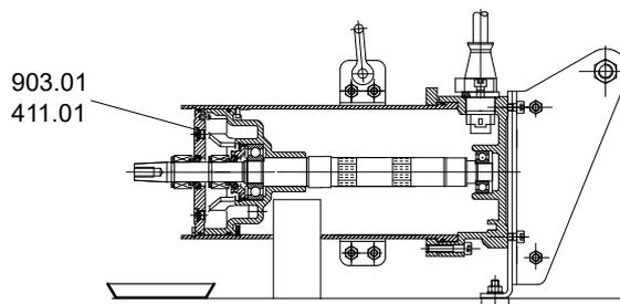
**Fig. 11:** Topping up the lubricant
