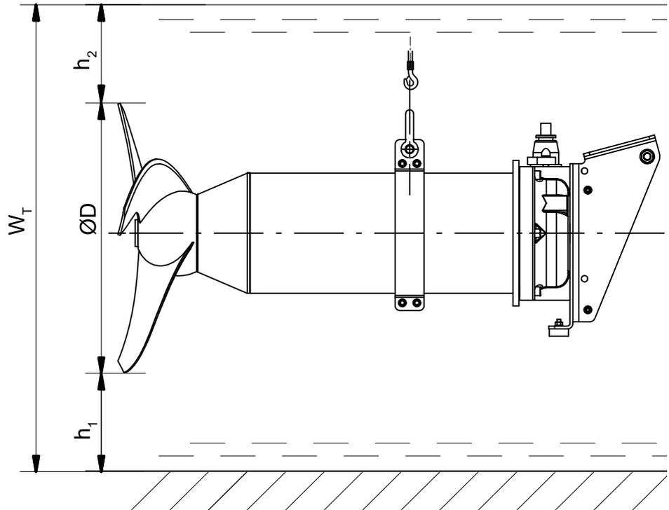
Fig. 9: Minimum level of fluid handled
