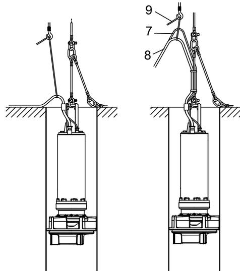
**Fig. 13:** Securing the control and power cables
