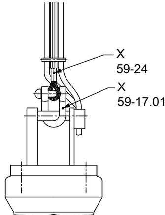
Fig. 10: X = indication of load-carrying capacity
