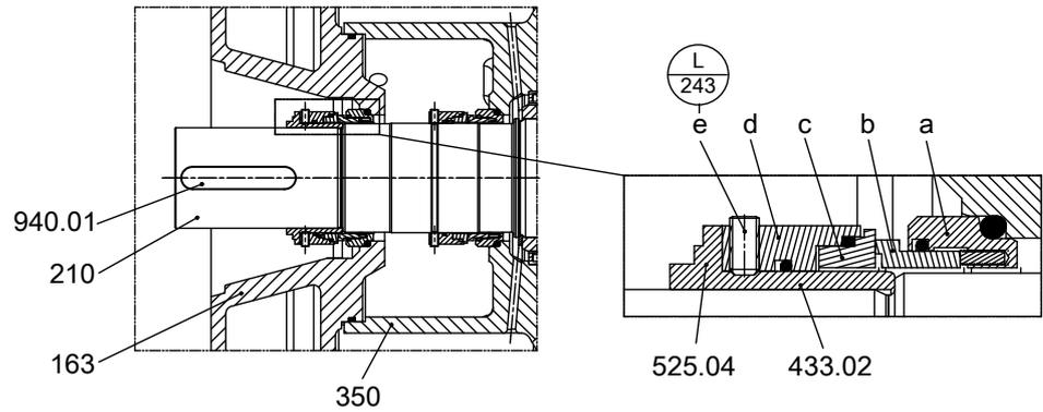
Fig. 45: Installing the impeller-end mechanical seal for motors 320 6.N, 360 6.N, 400 6.N, 440 6.N
