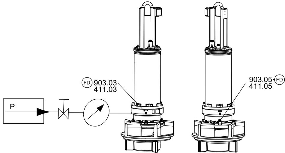
**Fig. 50:** Leak testing the lubricant reservoir
