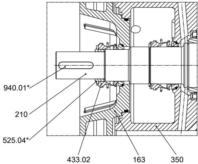
**Fig. 34:** Drawing of the impeller-end mechanical seal for motors 95 4.N, 60 6.N, 80 6.N, 100 6.N, 120 6.N, 140 6.N, 165 6.N, 190 6.N, 225 6.N, 260 6.N, 90 8.N, 110 8.N., 130 8.N, 150 8.N, 185 8.N, 40 10.N, 60 10.N, 75 10.N
