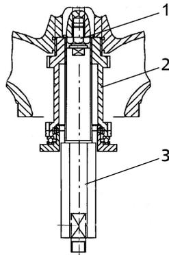
**Fig. 33: Special impeller fitting and removal tool**
