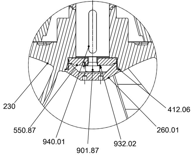
Fig. 69: Impeller fastening elements, sizes 1000-420, 1000-421, 1000-500, 1200-630
