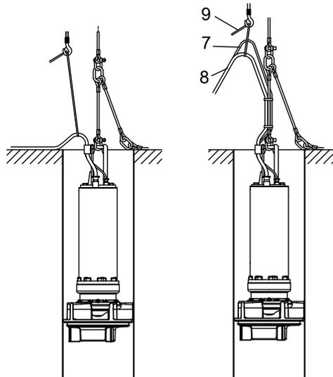
**Fig. 19:** Securing the control cable and power cables
