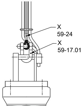
Fig. 16: X = indication of load-carrying capacity
