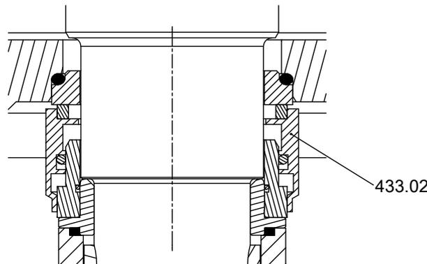
**Fig. 82:** Mechanical seal with covered spring, optional for motors 95 4.N, 60 6.N, 80 6.N, 100 6.N, 120 6.N, 140 6.N, 165 6.N, 190 6.N, 225 6.N, 260 6.N, 90 8.N, 110 8.N., 130 8.N, 150 8.N, 185 8.N, 40 10.N, 60 10.N, 75 10.N
