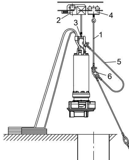
**Fig. 18:** Lifting and positioning the pump set
