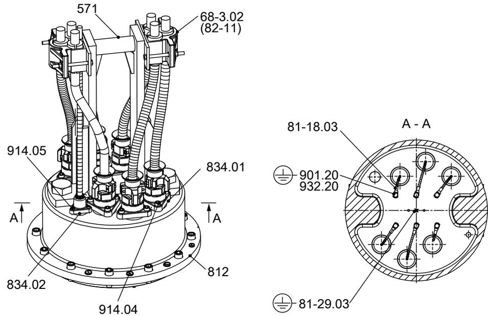
Fig. 39: Removing the connection cable and cable gland
