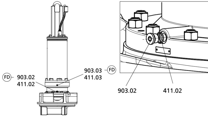
Draining the leakage
