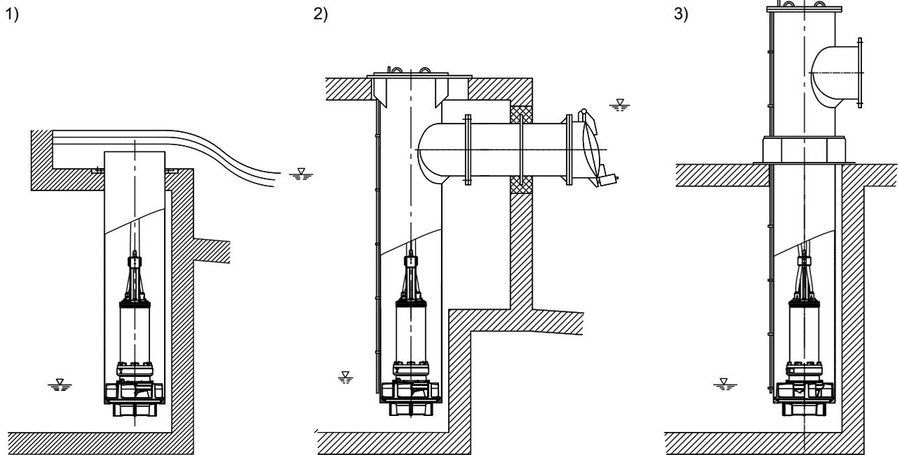
Fig. 5: Overview of installation types
