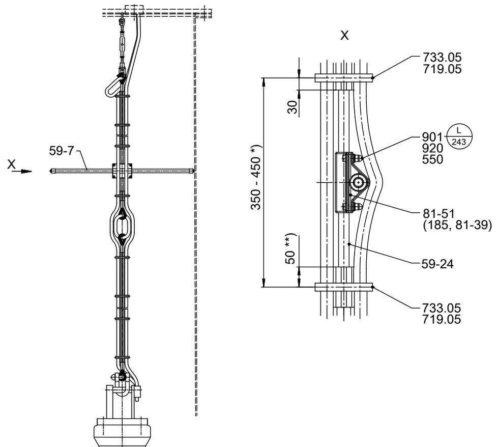
**Fig. 21:** Support rope with support, dimensions in [mm]
