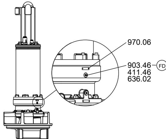
Fig. 29: Lubricating nipple
