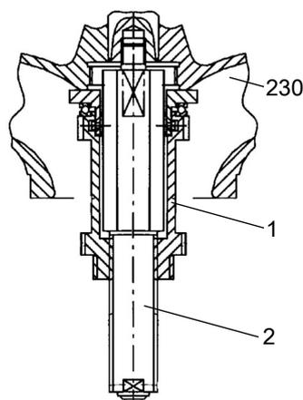
**Fig. 47:** Special impeller fitting and removal tool
