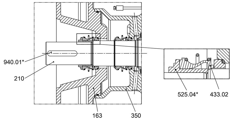
**Fig. 44:** Installing the impeller-end mechanical seal for motors 95 4.N, 60 6.N, 80 6.N, 100 6.N, 120 6.N, 140 6.N, 165 6.N, 190 6.N, 225 6.N, 260 6.N, 90 8.N, 110 8.N., 130 8.N, 150 8.N, 185 8.N, 40 10.N, 60 10.N, 75 10.N
