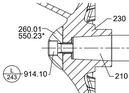
Fig. 68: Impeller fastening elements, sizes 700-330, 800-400, 800-401
