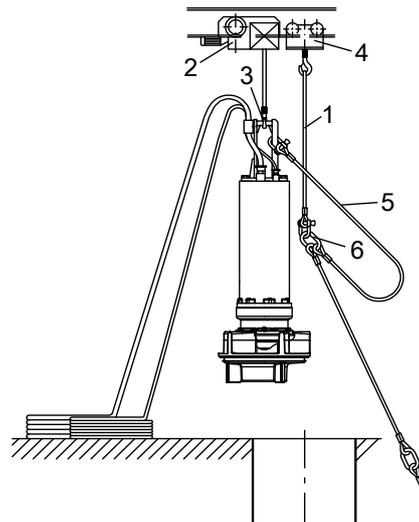
**Fig. 12:** Lifting and positioning the pump set
