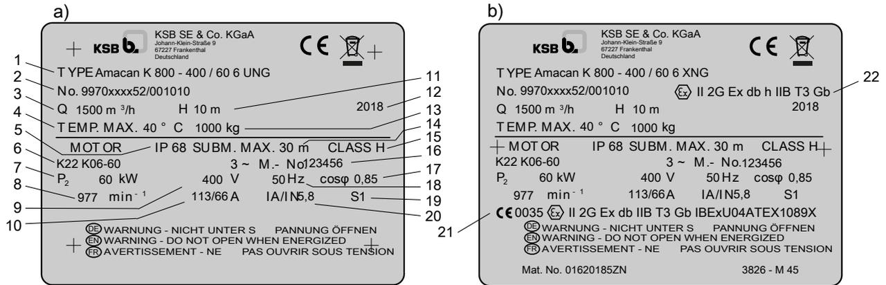
Fig. 4: Name plate (example) a) Standard pump set b) Explosion-proof pump set
